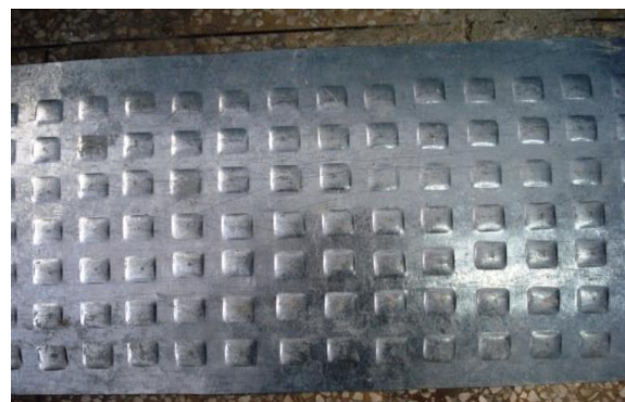
Figure 2: Photographic View of Absorber Plate Roughened by Formation of Square Protrusions
